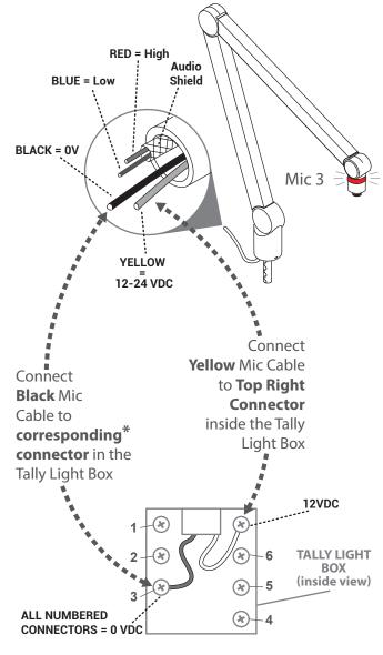
\* See label inside Tally Light Box Cover to choose a numbered connector according to Mic No.
